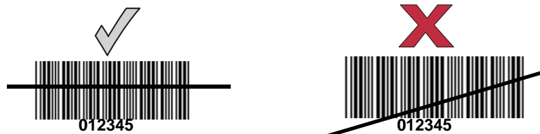
Figure 2-3 Acceptable and Incorrect Aiming
